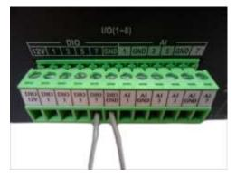
5. Configure the DIO ports in Web Configurator (see the Encoder Firmware Manual for more information).
