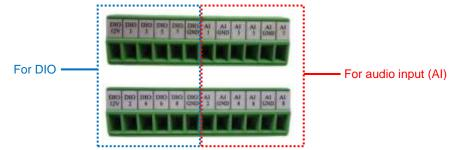
To connect an audio input device, do the following:
