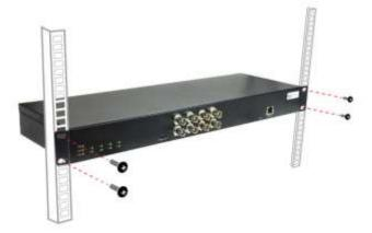
**NOTE:** Use the screws that came with the rack; or, purchase applicable screws for rack mounting.
