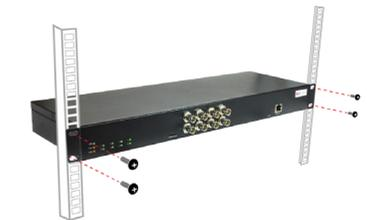
**Note:** Use the screws that came with the rack; or, purchase applicable screws for rack mounting.
