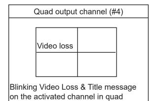
The warning message and the buzzer can be cleared by pushing Lock button (#2) for more than 4 seconds if the device is operated under Security lock On mode, or pushing any button on the front panel if the device is operated under Security lock OFF mode.
