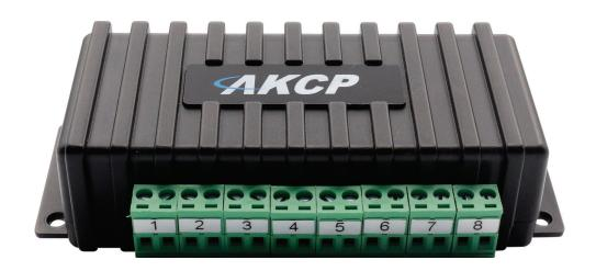
The IO-digital8 sensor adds 8 dry contacts to the securityProbe or expansion module base unit. With 8 ALARM/NORMAL indication in the web interface it provides instant notification for changes of status.
