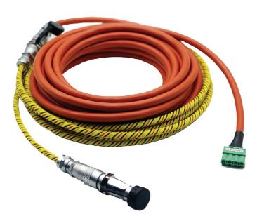
The rope water sensor comes in two parts, the orange non-sensing cable, and the yellow sensing cable. IP66 rated waterproof connectors join the sections of rope together, with an additional connector at the tail end allowing the sensor to be extended with additional lengths as required. Lay these rope water sensors out around the perimeter of your room, or underneath aisles in your data center to give early warning of potential water leaks and avoid costly damage.
