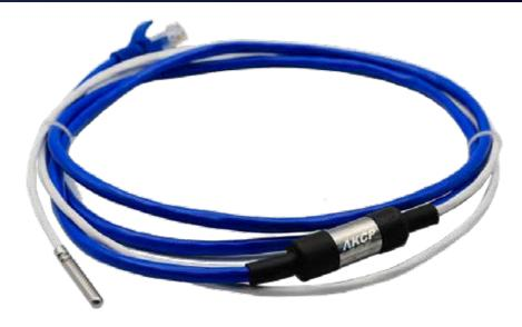
Suitable for temperatures as low as -200°C (-328°F). Ideal for monitoring vaccines and medical products based on mRNA technology that require ultra cold storage. The sensor uses a platinum probe that varies in resistance with temperature changes.
