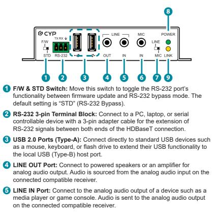
6 MIC IN Port: Connect to a standard unpowered microphone using a 3.5mm plug.
