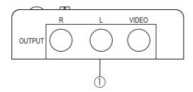
① OUTPUT R/L/VIDEO: These slots are to connect with output display TV/monitor with R/L & composite RCA jack cable.
