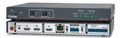
The Extron DTP2 T 212 is a two-input transmitter for sending HDMI, audio, and control up to 330 feet (100 meters) over a shielded CATx cable to an Extron DTP®-enabled product. It provides two HDMI inputs, one DTP2 output, and one HDMI output. It supports video resolutions up to 4K/60 at 4:4:4 chroma sampling, and complies with HDCP 2.2. With several integrator-friendly features in a low-profile enclosure, the DTP2 T 212 enables discreet installation in a wide variety of applications.
