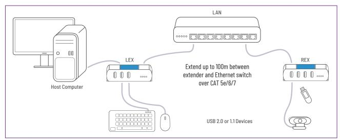
\* Maximum throughput will vary based on network traffic, distances and number of switches between extenders. \*\* Pre-paired network configuration only applies to units purchased together as a complete LEX and REX extender system.
