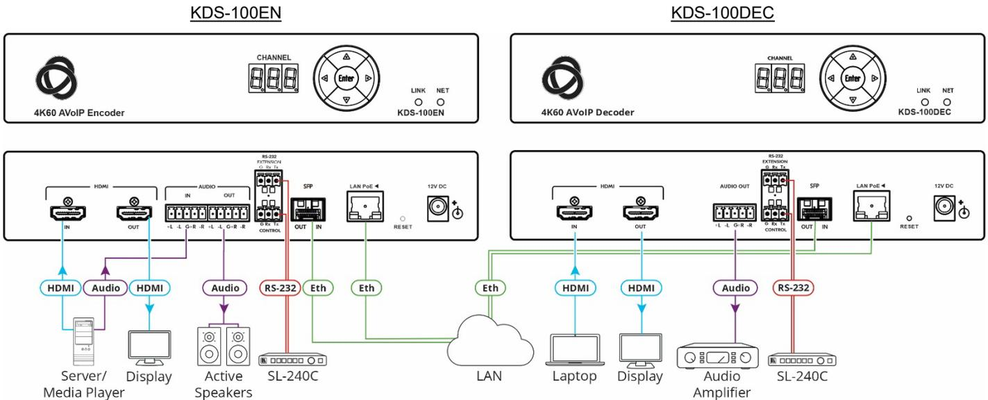
**KDS-100EN** and **KDS-100DEC** can stream 4K video, requiring a gigabit Ethernet switch for high quality performance, while the maximum momentary transfer rate can reach 60Mbps. We recommend using AVoIP Ethernet switches that support: PoE+, multicast forwarding or filtering, IGMP Snooping, IGMP Querier and IGMP snooping fast leave.
