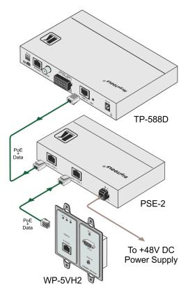
Figure 3: Connecting the PSE-2 10Gb POE Injector
