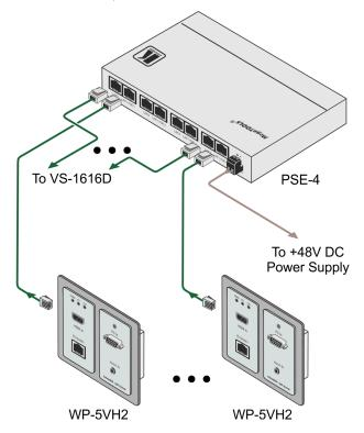
Figure 3: Connecting the PSE-4 10G Quad POE Injector
