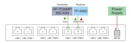
Figure 4: The PSE-4 Supplying Power to Receivers
