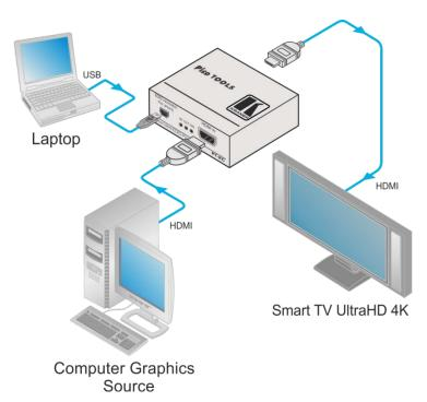
Figure 2: Connecting the PT-2C Extended EDID Processor
