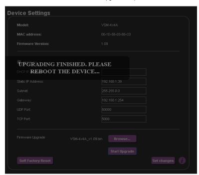
Figure 42: Device Settings Page - Firmware Upgrade Complete
