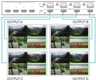
Figure 10: Connecting the VSM-4x4A in Quad Operation Mode
