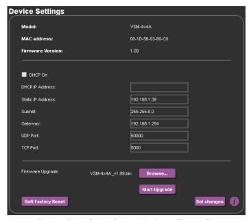
Figure 40: Device Settings Page - Uploading the Firmware File
