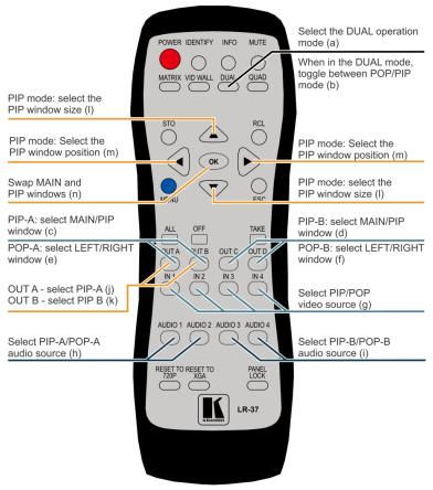
Figure 19: IR Remote Control Transmitter Dual Mode Shortcuts
