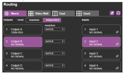
Figure 22: Matrix Tab output Resolution (Independent Mode)
