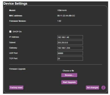
Figure 37: The Device Settings Page – Ethernet Settings
