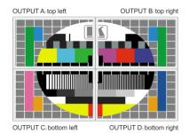
Figure 4: VSM-4x4A Video Wall Operation Mode
