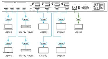
Figure 3: Connecting the VSM-4x4A Presentation Switcher / Scaler
