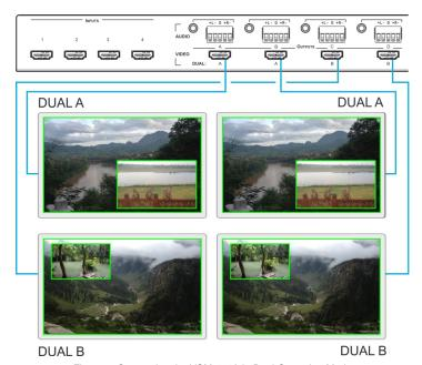
Figure 8: Connecting the VSM-4x4A in Dual Operation Mode
