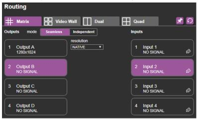
Figure 21: The Matrix Tab output Resolution (Seamless Mode)
