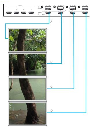
Figure 6: Connecting the VSM-4x4A in 1x4 Video Wall Operation Mode
