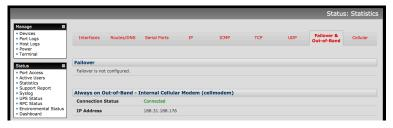
> At any time you may view the cellular signal strength (**RSSI**) from the **Cellular** tab of the **Status: Statistics** page — an RSSI of -100 dBm and less is unacceptable coverage, -99 to -90 is weak to medium coverage, -89 to -70 is medium to strong coverage, -69 and greater is very strong coverage
