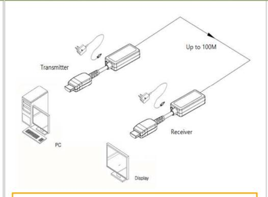
**NOTE**: The Transmitter and Receiver modules must be connected to the included power supplies (5V DC) for proper operation.
