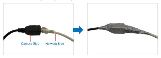
**NOTES on using Ethernet cables:** For outdoor installations, it is recommended to use *exterior-grade* Ethernet cables (CAT5/CAT5e/CAT6); ordinary Ethernet cables are only designed for indoor use and may deteriorate quickly when exposed to outdoor elements. Exterior-grade Ethernet cables are waterproof and do not require a conduit.
