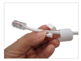
23. Insert the cable through the gland body.
