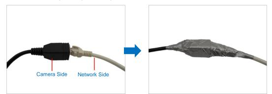
**NOTES on using Ethernet cables:** For outdoor installations, it is recommended to use *exterior-grade* Ethernet cables (CAT5/CAT5e/CAT6); ordinary Ethernet cables are only designed for indoor use and may deteriorate quickly when exposed to outdoor elements. Exterior-grade Ethernet cables are waterproof and do not require a conduit.
