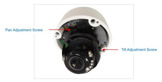
**NOTE**: Be careful when turning the lens module to its extent as cables are connected inside the module.
