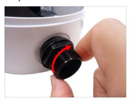
4. Pull the network cable through the flex conduit. If connecting other input/output devices or an external power adapter, pull the cables through the flex conduit without connectors. The terminal blocks will be attached once the cables pass through the camera hole later.
