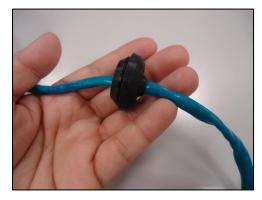
4. Once the Ethernet cable passes through the camera hole, attach the RJ-45 connector (see *How to Attach the RJ-45 Connector* on page 32 for detailed information).
