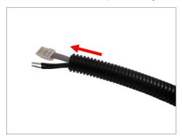
5. Insert the clamping nut through the flex conduit.
