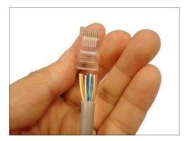
6. Place the connector into the crimping tool, and cinch down to secure the RJ-45 connector to the Ethernet cable.
