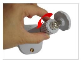
3. Screw the camera to the bracket.
