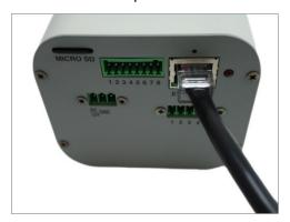
2. If necessary, connect the other external devices, such as DI/DO, PT scanner or power adapter to the camera. See *Before Installation* on page 15 for more information.
