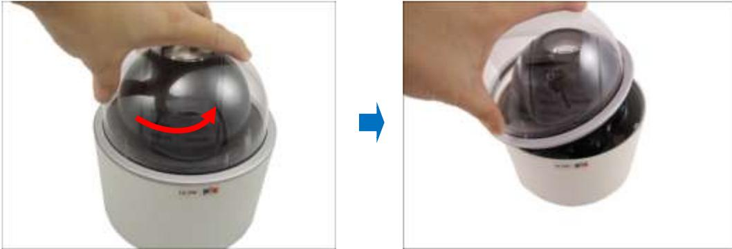
2. Rotate the replacement dome cover clockwise to attach it.
