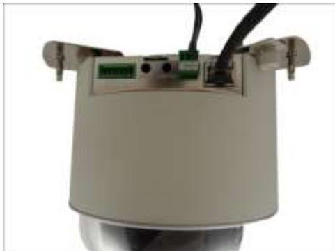
**NOTE:** The cables may be routed along the ceiling if the camera is installed on a hard ceiling. Or, the cables may pass through a hole on the ceiling if the camera is installed on a dropped ceiling.
