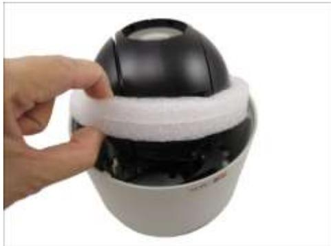
3. Rotate the dome cover clockwise to attach it.
