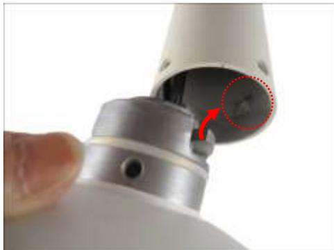
3. Twist the mount kit to align the screw holes and attach the two (2) mounting screws (included in the mount kit package).
