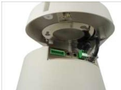
2. Align and insert the camera base hooks to the mounting holes.
