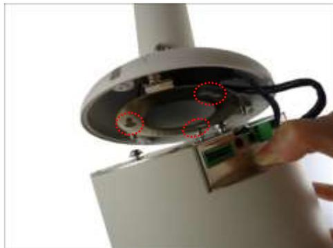
3. Slide the camera counter-clockwise to secure the hooks to the mount.
