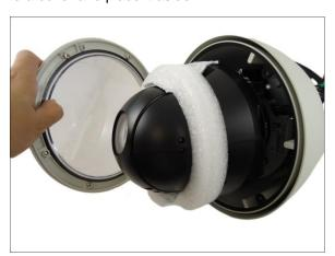
**NOTE:** The cover is attached to the camera by a metallic wire strap; do not abruptly lift the cover.
