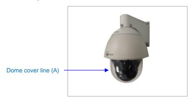
NOTE: A blurry image may result when the lens is tilted along or above the line on the dome cover (A).
