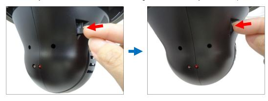
5. Align the screw holes and tightly secure the screws using the bundled hex screwdriver.
