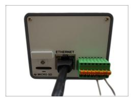
3. Connect the other end of the network cable to a switch or injector. Then, connect the switch or injector to a network, PC and a power source. See Power-over-Ethernet (PoE) connection example below.
