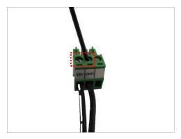
5. When ready, connect the prepared power adapter to the **POWER** connector of the camera. Below is an example of a power adapter with an attached terminal block.
