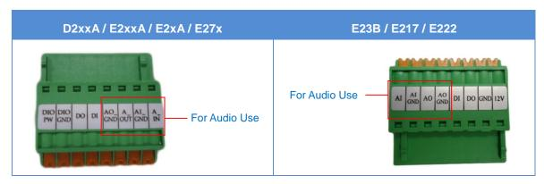
2. To connect audio devices, map the pins to one of the pin combinations below:
