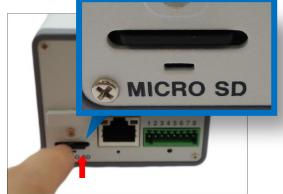
To avoid unauthorize removal of the card, cover the memory card slot. To do this, loosen the screw and turn the tab to cover the memory card slot. Once the tab is in place, tighten the screw.
