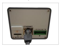
If necessary, connect audio input/output or DI/DO devices to the camera. See How to Connect DI/DO and Audio Devices on page 25 for more information.
