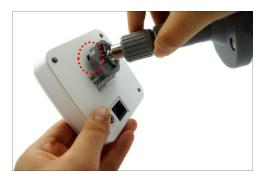
2. Tighten the knob to fix the camera.
