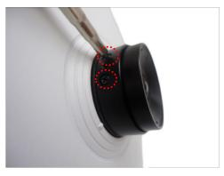
Proceed to adjust the camera viewing angle and focus (see Step 6: Adjust the Viewing Angle and Focus on page 12 for more information).
