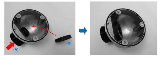
2. Insert the Ethernet cable through the back cover and then align the sealing insert to the gland body.
