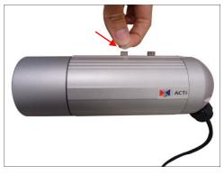
2. Attach the sunshield then loosely secure it with the supplied screws.
