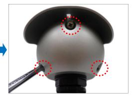
**CAUTION:** Make sure the rubber seal is properly attached and the back cover is closed to ensure water or dust cannot enter the camera.
