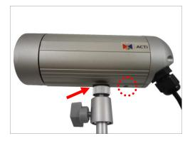
2. Adjust the camera viewing angle and tighten the knob to fix the camera position.
