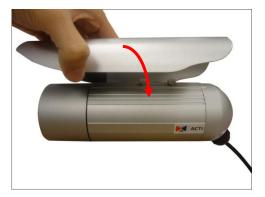
3. Slide to adjust the sunshield to cover the lens as far as possible but out of the camera's live view.
