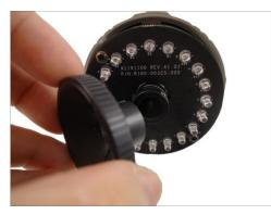
Adjust the focus of the target area, based on the live view of the camera (see Access the Camera on page 35).
