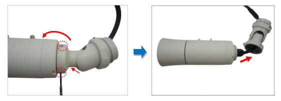
2. Loosen the three (3) screws securing the back cover and open the back cover.
