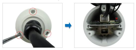
NOTE: Cables are connected inside the camera, do not abruptly pull the back cover.
