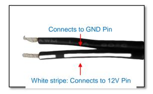
Connect the wire with the white stripe to the 12V pin and the other to the GND pin.
