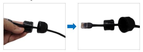
4. Attach one (1) supplied rubber ring on the gland body (smooth end).
