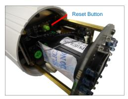
NOTE: DO NOT remove the desiccant bag inside the camera to keep the interior parts dry.
