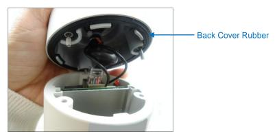
**NOTE:** Ensure that the rubber is properly aligned to the cover when closing the back cover.
