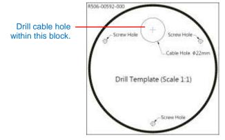
3. Route the cable from the network side through the hole and connect it to the Ethernet port of the camera.
