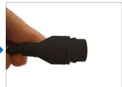
2. Detach the clamping nut from the cable gland:
