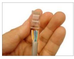
6. Place the connector into the crimping tool, and cinch down to secure the RJ-45 connector to the Ethernet cable.
