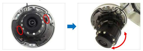
4. To rotate the video orientation, turn the lens module left or right.
