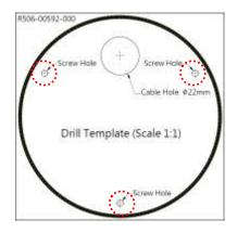
3. Drill the screw holes. Depending on the material of the surface where the camera will be installed, it may be necessary to drill the three (3) screw holes and use the supplied screw tox.
