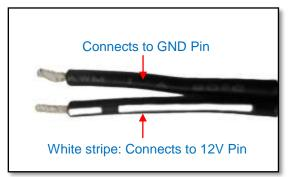
3. Connect the wire with the white stripe to the **12V** pin and the other to the **GND** pin.
