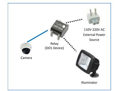
The illustration below is a graphic example of connecting a relay to a high voltage DO device.
