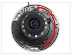
3. To tilt the lens, loosen the two (2) tilt adjustment screws. Then, adjust the tilt and tighten back the screws to fix the tilt position.
