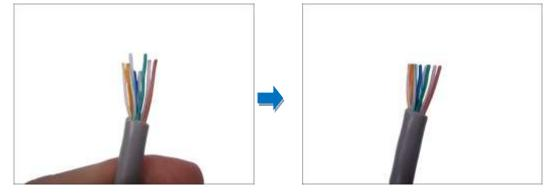
5. With the RJ-45 connector tab facing down, push down the wires into the connector all the way to the end.
