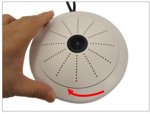
4. Remove the thin film protecting the lens.
