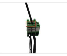
5. Set the prepared power adaptor for connection later. Below is an example of a power adaptor with an attached terminal block.
