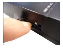
Once inserted, make sure to access the camera Web Configurator and "mount" the card to prepare the card for local recording. Refer to the camera Firmware User's Manual for more information.
