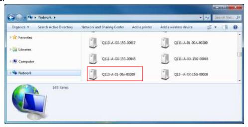
Double-click the mouse on the camera model name, the default browser of the PC is automatically launched and the IP address of the target camera is already filled in the address bar of the browser.
