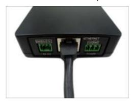
2. Connect the other end to a switch or injector. Then, connect the switch or injector to a network or PC and a power source. See Power-over-Ethernet (PoE) example connection diagram below.
