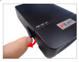
2. Insert the memory card with the metal contacts facing down the main unit.
