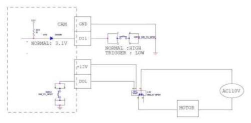
Note that when choosing an appropriate relay, please refer to its specifications and make sure they match the above design. The triggering circuit voltage has to be around 12V DC and the switch-controlled circuit voltage has to match the external power supply (e.g. 110V AC or 220V AC).
