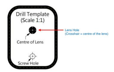
3. After drilling the lens hole, remove the drill template.
