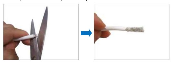
5. Twist the braid or tinned copper wires together and remove the foil coating.
