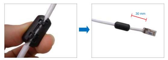
**NOTE:** The ferrite core is used to suppress electromagnetic interference (EMI) from the camera that may affect other devices, as well as prevent the EMI from other electronic devices to affect the performance of the camera.
