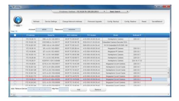
You can quickly notice the camera model in the list. Click on the IP address to automatically launch the default browser of the PC with the IP address of the target camera already filled in the address bar of the browser.
