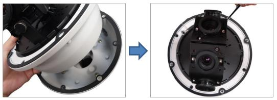
Adjust the camera tilt and viewing angle to complete the installation, see *Adjust Camera Tilt and Viewing Angle* on page 23.
