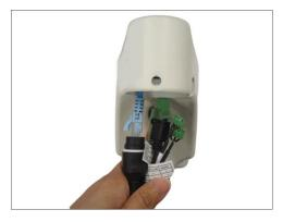
**CAUTION:** The camera itself is waterproof, however take note that the cable connections are not. If the cable connections will be exposed outdoors, make sure to shield or adapt proper waterproofing methods. See *Waterproof the Cable Connections* on page 19.
