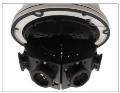
3. Move the module base to pan the camera.
