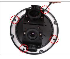
3. Lift the camera module and pull out the cables through the mount kit and housing.
