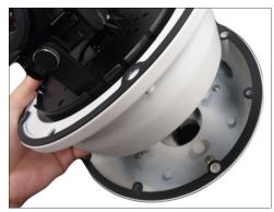
4. Remove the four (4) screws securing the mount kit to the housing, and then detach the mount kit.
