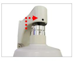
2. Attach the two (2) screws included in the wall mount package to secure the camera.
