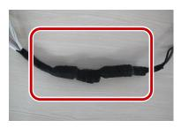
Choose a start point for waterproof tapes and protect the tail cables using waterproof tapes.
