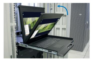
■ Flip up the LCD to a suitable angle.
