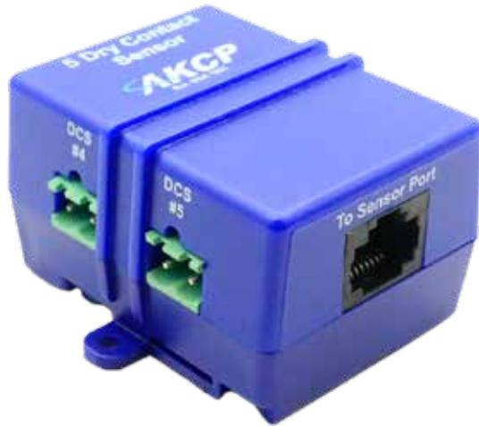
The single port RJ-45 Dry Contact Sensor with an ALARM/NORMAL indication in the software. Can have up to two on a SP2, four on an SP2+ eight on a SP8 and 600 Dry Contact Sensors on a securityProbe unit. Dry contact sensors are user definable and can be used to detect many different inputs such as UPS status, security systems, air conditioning status.
