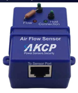
The airflow sensor is a switch type on/off style sensor. It is not a precision airflow measurement sensor, but rather an indicator of whether there is a presence or absence of airflow. A threshold can be set to determine the sensitivity of the sensor. Ideal for placing in-front of air intake or exhaust fans to indicate if the airflow is sufficient and as an early warning of failures in the cooling sytems or fans.
