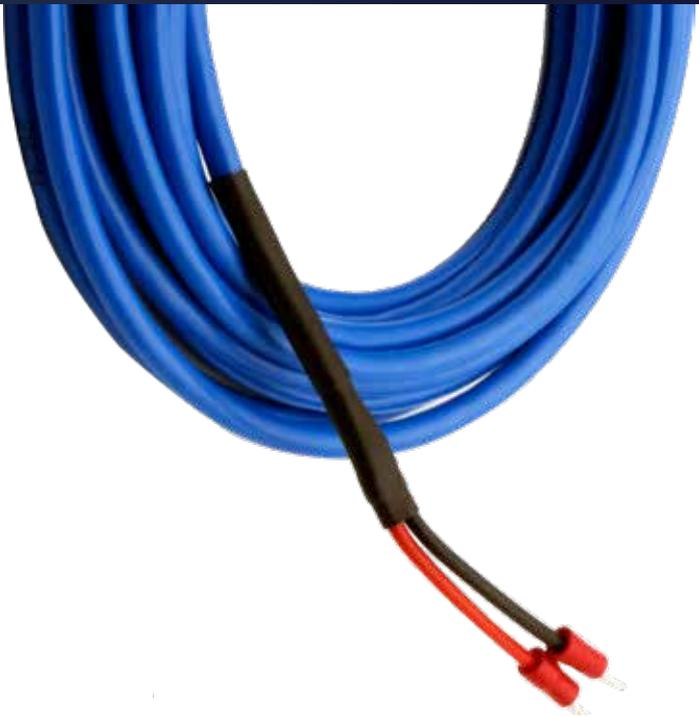
The Dry Contact sensor is a simple connection to burglar alarms, fire alarms or any application that requires monitoring by the sensorProbe. Dry contact sensors are user definable and can be used to detect many different inputs such as UPS status, security systems, air conditioning status.
