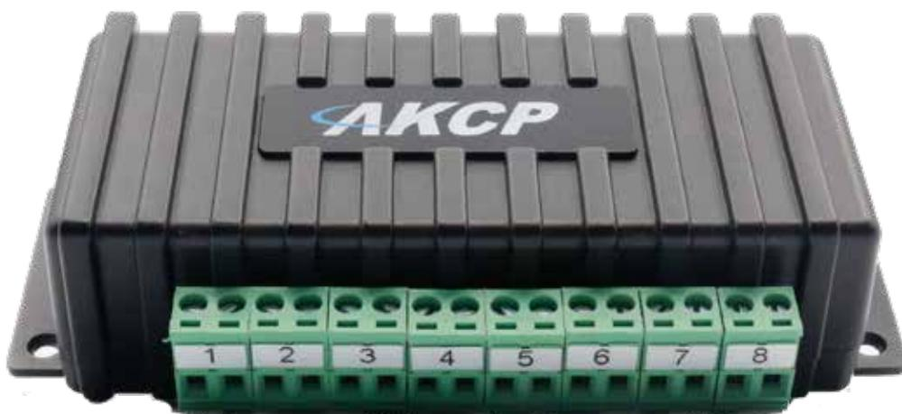
The IO-digital8 sensor adds 8 dry contacts to the securityProbe or expansion module base unit. With 8 ALARM/NORMAL indication in the securityProbe 5E web interface it provides instant notification for changes of status. The sensor can be mounted on a wall by your alarm panel, or using our DIN rail clips can be DIN rail mounted. A standard CAT5 cable connects the IO-digital8 sensor to the intelligent sensor port.
