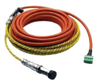
The rope water sensor comes in two parts, the orange non-sensing cable, and the yellow sensing cable. IP66 rated waterproof connectors join the two sections of rope together. Lay these rope water sensors out around the perimeter of your room, or underneath aisles in your data center to give early warning ofpotential water leaks and avoid costly damage.
