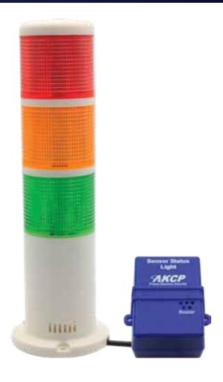
Connect the Sensor Status Light to any SPX+ or SP2+ sensor port. The light will change color based on a sensor status. Ideal for systems and control, factory automation and data center applications. Use as part of the Rack+ system to easily identify which cabinets in your data center are in a warning or critical state.
