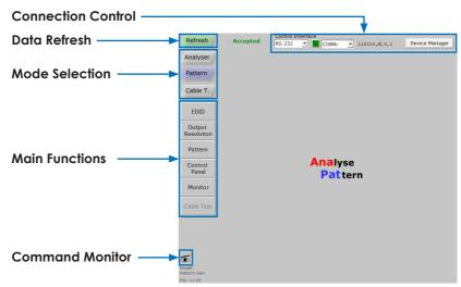
Figure 1: Mode Selection, Portable Version
