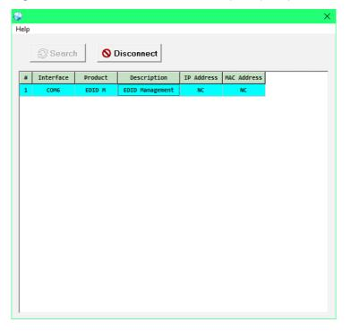
After launching the software, power the unit on and then connect it to the PC/laptop using a USB cable. Click on the "Search" button and any detected units will be displayed in the list. Clicking on a detected unit will open the EDID Commander window.
