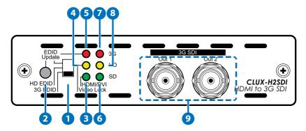
1 EDID Switch: Use this switch to select between the built-in or to update the EDID settings. Default EDID settings as shown below:
