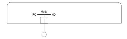
(1). PC/HD switch: This slide switch allows you to select PC or component HD timing output. Simply slide the dip switch to left or right and the output mode will display your desire selection.
