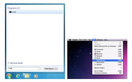
Once in the command line interface (CLI) type "telnet", then the IP address of the unit and hit enter.
