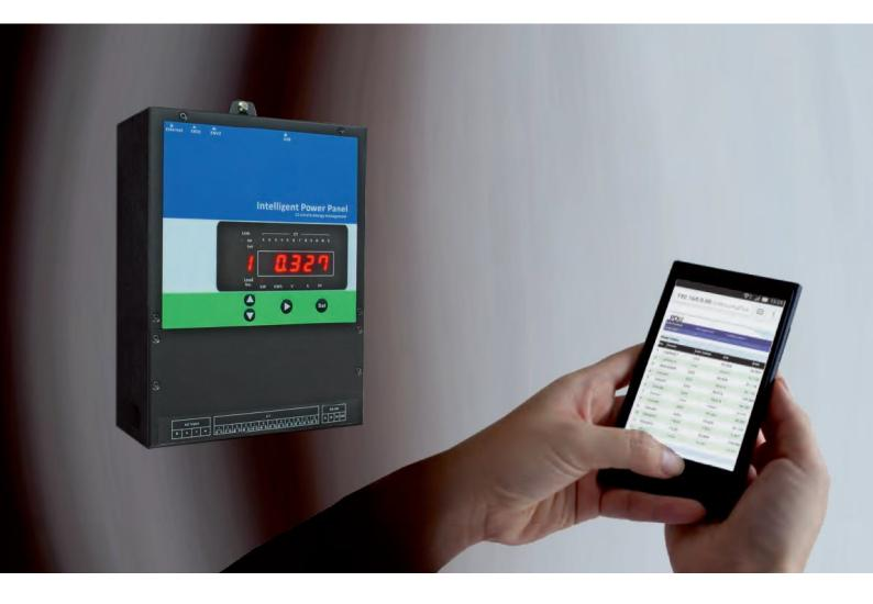
IPP series is a single/three phase remotely monitored power meter, built-in 12 independent measurement modules. User may select any one phase of the input voltage as a measurement reference. It supports the monitoring of twelve loops of 1P2W, or four loops of 3P3W/3P4W, or a hybrid combination, providing flexible application.
