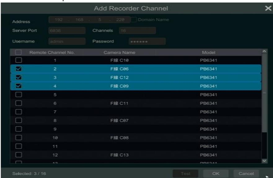
**Note :** Only the local NVR has unoccupied channels, may the IPC of other NVR/DVR in the same local network be added. And the added IPC supports previewing and recording.
