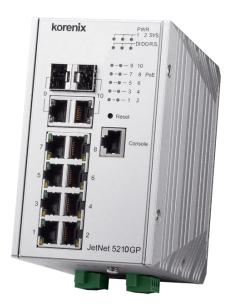
Korenix JetNet 5210GP, the DIN-Rail type industrial Gigabit Managed PoE Switch is designed with eight 10/100/1000TX ports, two Gigabit RJ-45 / SFP combo ports. JetNet 5210GP is the first industrial ethernet switch compliance with IEEE 802.3af/at/bt, each ethernet port can max supports 90W for PD, and total budget up to 480W <sup>'Note</sup>.
