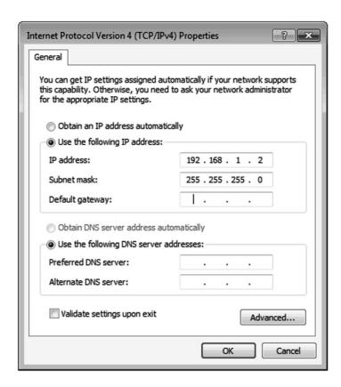
After successfully operating steps a. to h., you can click into Web UI by typing the 192.168.1.202 IP address in IE or Chrome.
