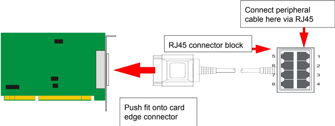
**Note:** The SPEED LE connector box cable needs to be secured or supported in case of sudden contact or excessive weight on the cables. Please ensure that adequate caution is taken to avoid possible damage to the SPEED LE card or Host system. This can be accomplished by securing the cable to a rack or to the back of the server.
