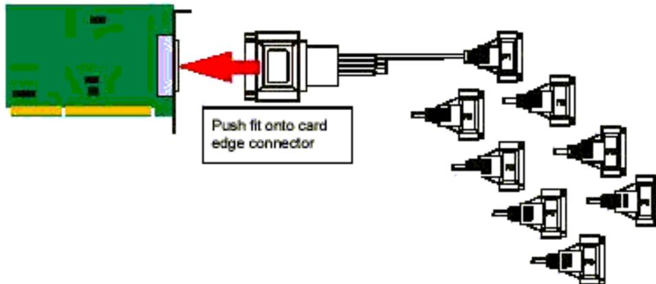
**Note:** The SPEED LE fan-out cables need to be secured or supported in case of sudden contact or excessive weight on the cables. Please ensure that adequate caution is taken to avoid possible damage to the SPEED LE card or Host system. This can be accomplished by securing the cables to a rack or to the back of the server.
