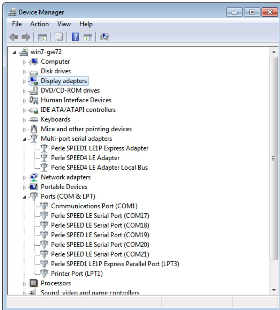
3. You can click on the **Multiport serial adapters** icon to display the currently installed devices. Each entry represents a SPEED LE card.
