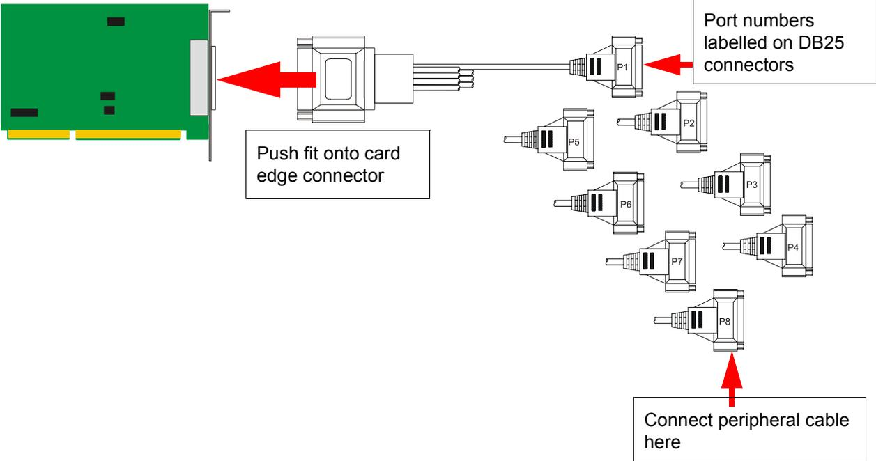
**Note:** The SPEED LE fan-out cables need to be secured or supported in case of sudden contact or excessive weight on the cables. Please ensure that adequate caution is taken to avoid possible damage to the SPEED LE card or Host system. This can be accomplished by securing the cables to a rack or to the back of the server.
