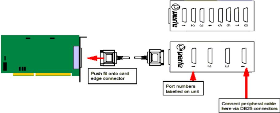
**Note:** The SPEED LE connector box cable needs to be secured or supported in case of sudden contact or excessive weight on the cables. Please ensure that adequate caution is taken to avoid possible damage to the SPEED LE card or Host system. This can be accomplished by securing the cable to a rack or to the back of the server.
