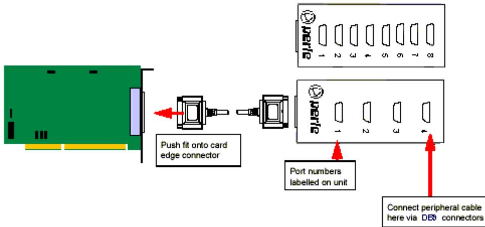
**Note:** The SPEED LE connector box cable needs to be secured or supported in case of sudden contact or excessive weight on the cables. Please ensure that adequate caution is taken to avoid possible damage to the SPEED LE card or Host system. This can be accomplished by securing the cable to a rack or to the back of the server.
