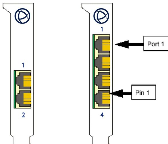
The RJ45 connector has a 10-pin configuration. If you require an 8-pin connector configuration, use the pinouts in the RJ45 8-pin column. The connector pinout for each RJ45 socket fitted to the SPEED LE Express cards is as follows;
