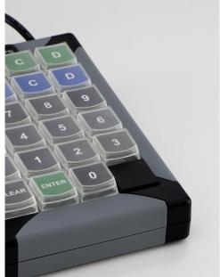
The Key Blocker should stay flat without the key plunger pushing up on it.
