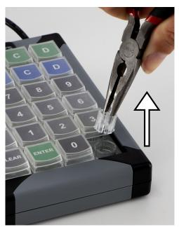
Using needle nose pliers, grip the stem of the Key Plunger and pull straight upward.
